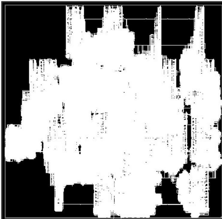
**Figure 4** – Routing of *cnv2d* Design Using the Soft 2D NoC
