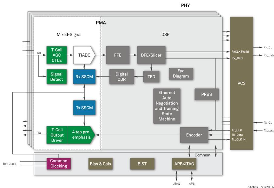
**Figure 4 • Speedster7t FPGA SerDes PHY Block Diagram**
