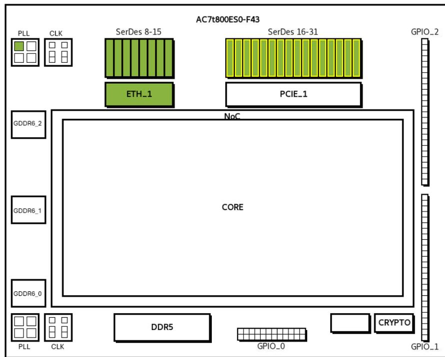
**Figure 3 • Speedster7t AC7t800 FPGA Top-Level Block Diagram**
