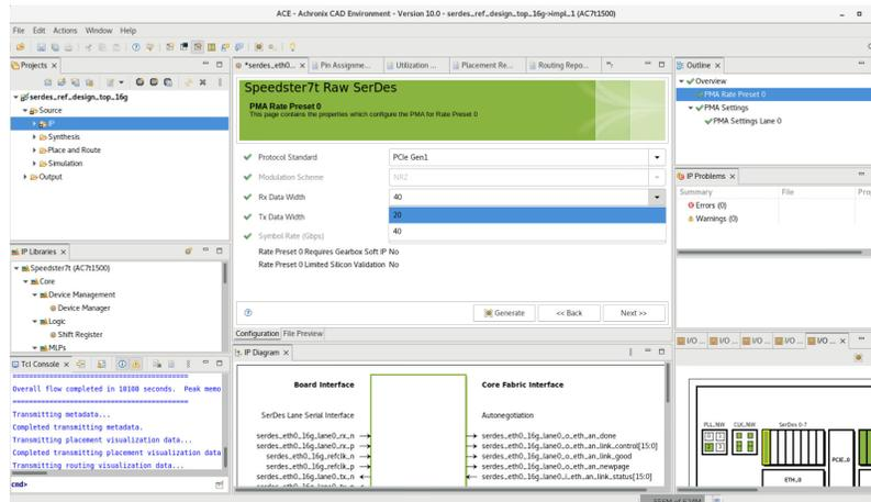
**Figure 20 • Setting the Receive and Transmit Data Widths**
