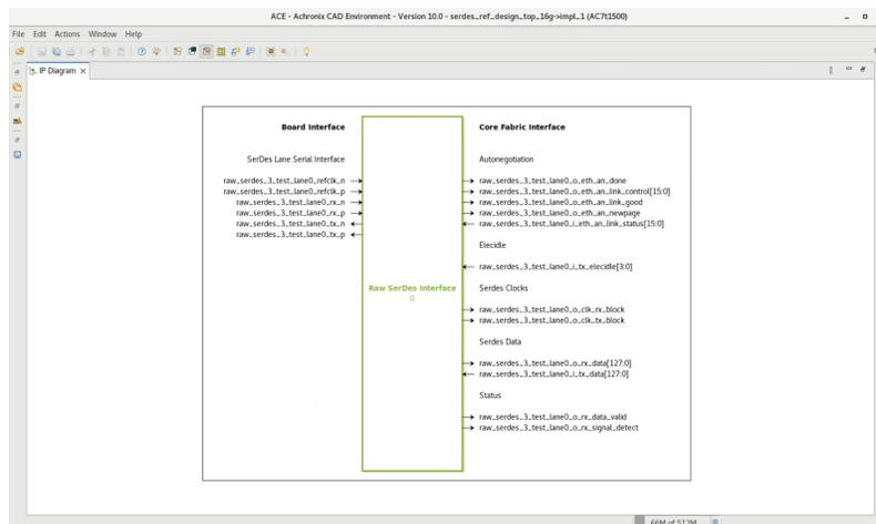
**Figure 24** • New IP Interface Pins and Signals.
