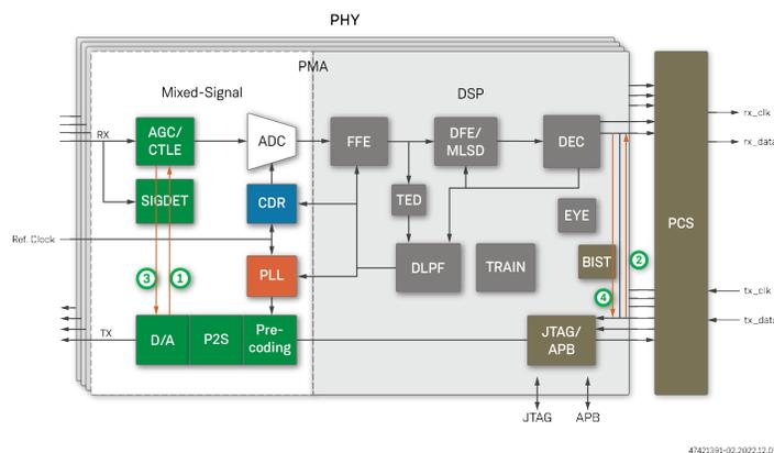
**Figure 5 • Speedster7t FPGA SerDes PHY Data Loopback Modes**
