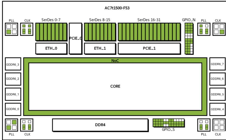
**Figure 2 • Speedster7t AC7t1500/AC7t1400 FPGA Top-Level Block Diagram**
