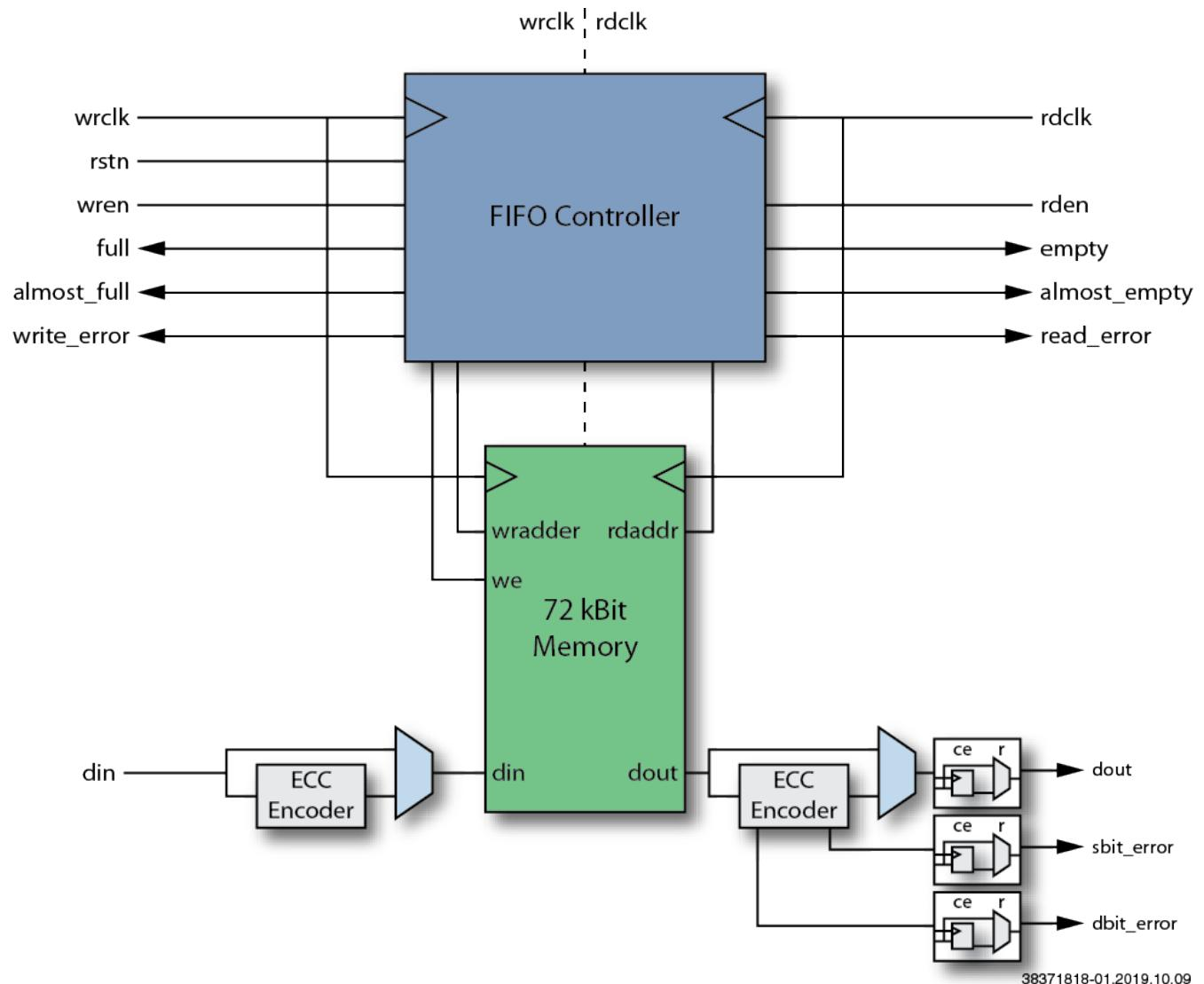
**Figure 62: BRAM72K\_FIFO Block Diagram**
