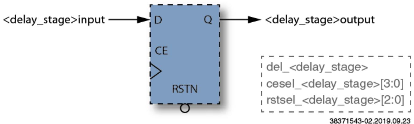
**Figure 40: Delay Stage Symbol**
