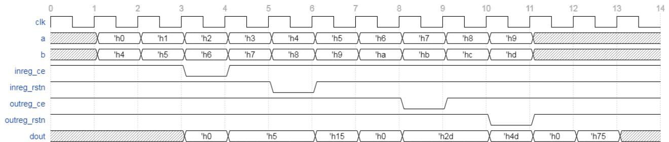
**Figure 51: Timing Diagram for Single Multiplier Channel**
