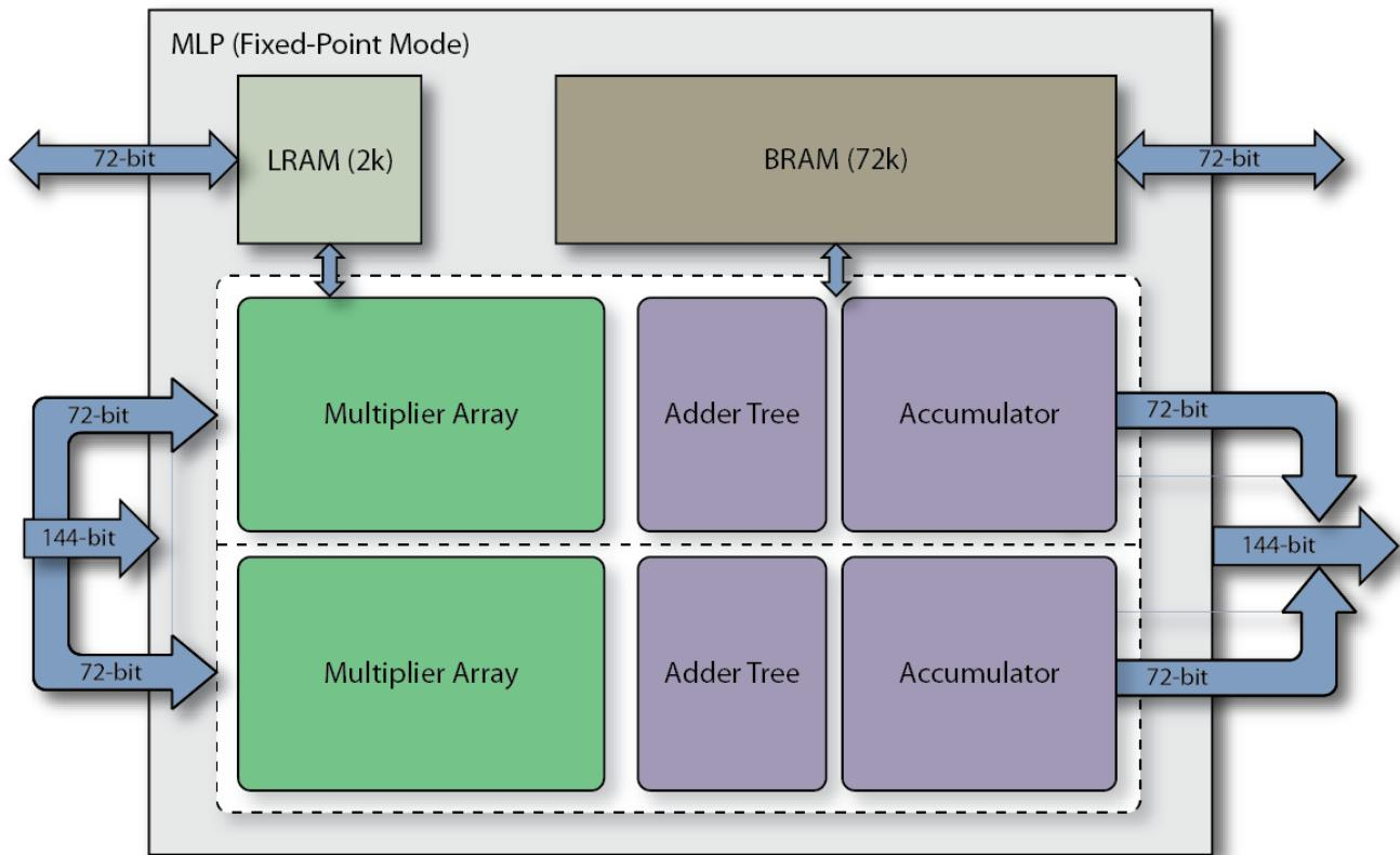
**Figure 36: MLP Using Fixed-Point Mode**
