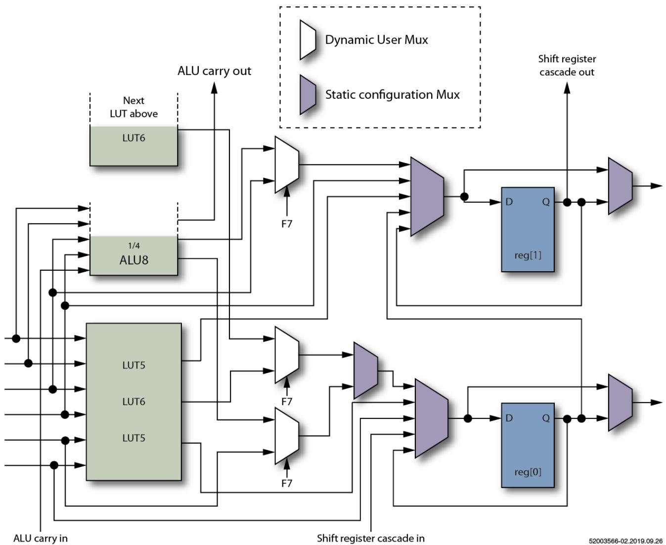
**Figure 6: One-Fourth of a Logic Group (Connection Detail)**
