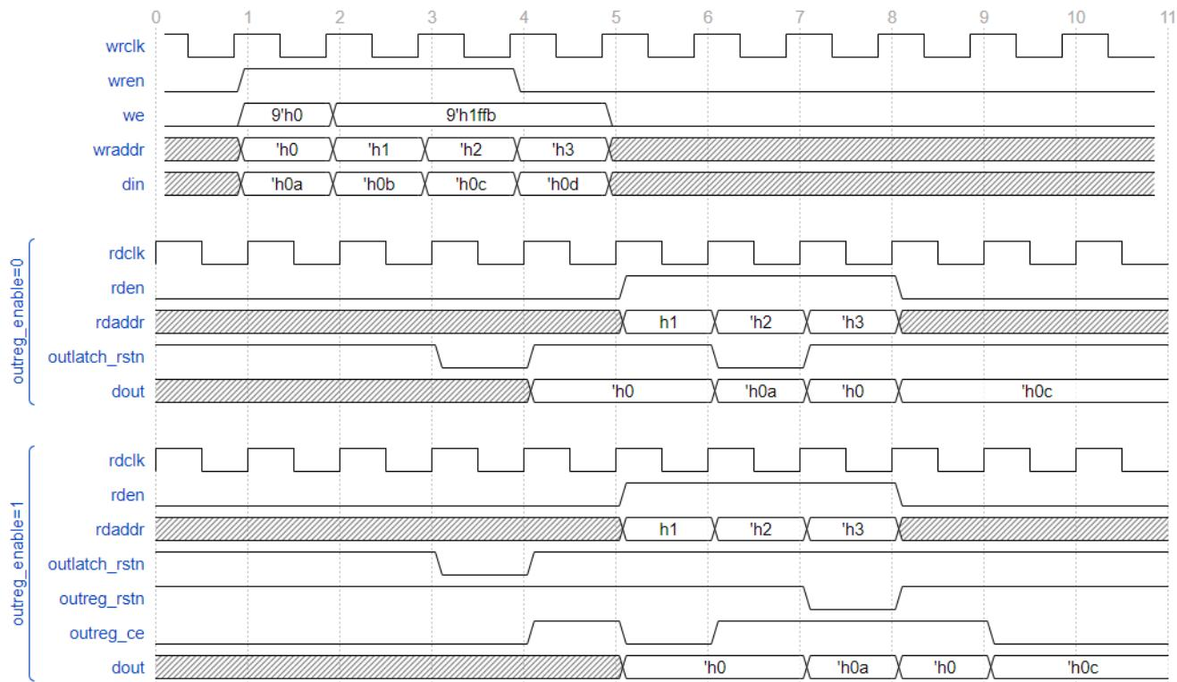
**Figure 65: BRAM72K\_SDH Timing Diagram**
