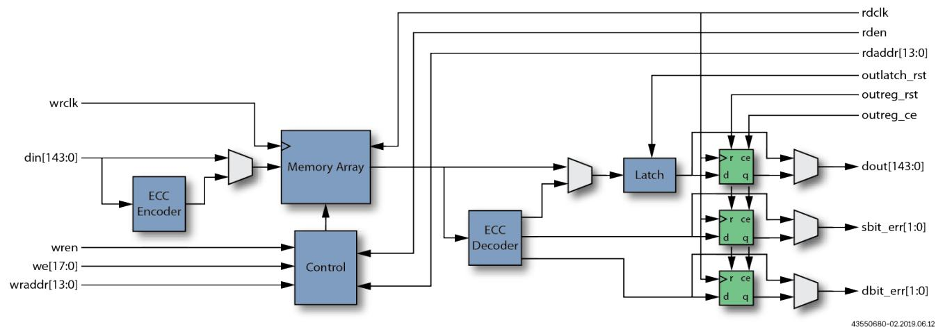
**Figure 64: BRAM72K\_SDPI Block Diagram**
