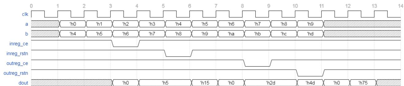
**Figure 53: Timing Diagram for a Single Multiplier Channel**
