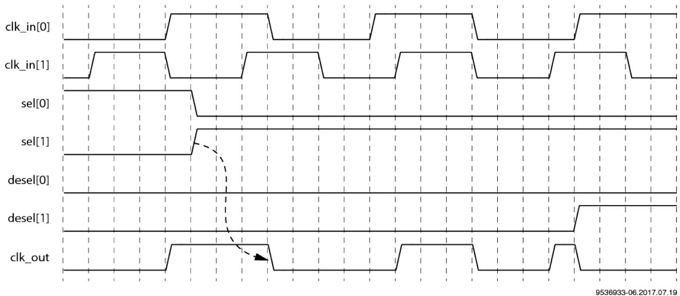
**Figure 34: SYNCHRONIZE\_SEL=0 Timing Diagram**
