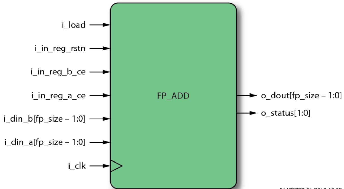
**Figure 54: Floating-Point Adder with Optional Accumulate**
