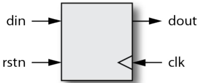
**Figure 25: ACX\_SYNCHRONIZER Logic Symbol**
