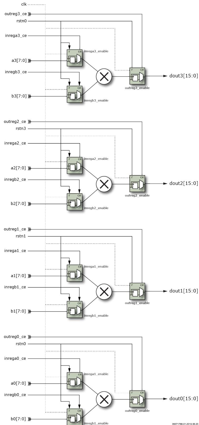
**Figure 50: MLP72\_INT8\_MULT\_4X Block Diagram**
