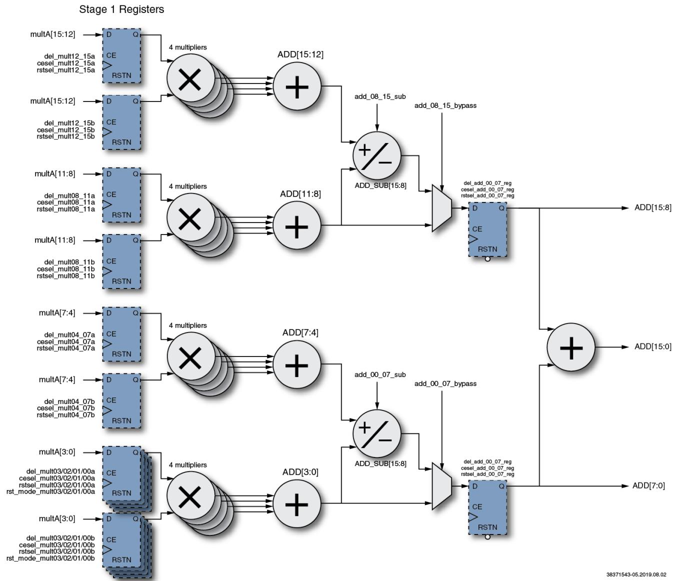
**Figure 43: Multiplication Stage Structure (Integer)**
