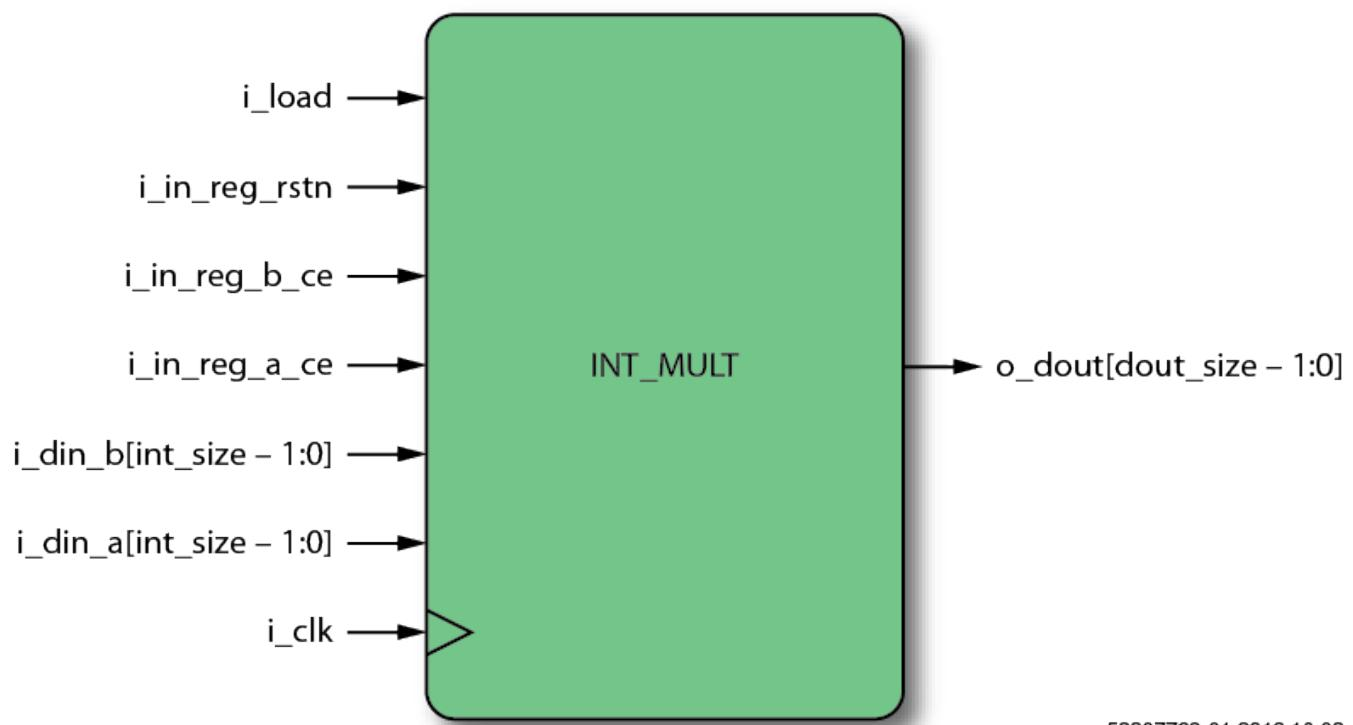
**Figure 59: Integer Multiplier with Optional Accumulate**
