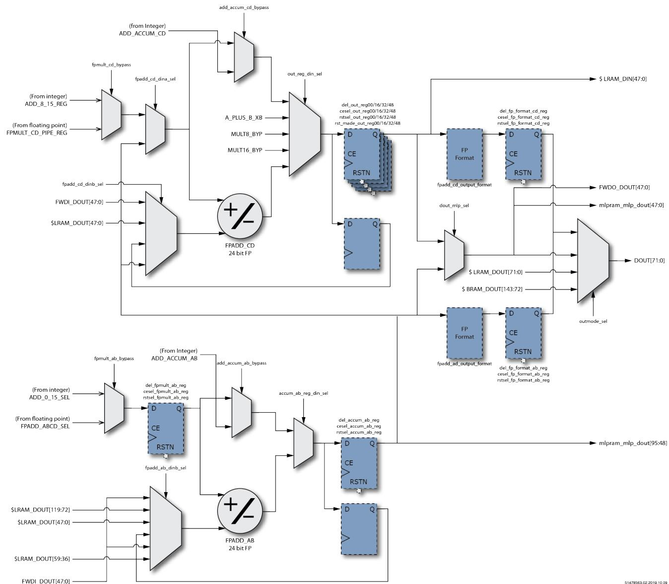
Figure 47: Floating-Point Output Stage
