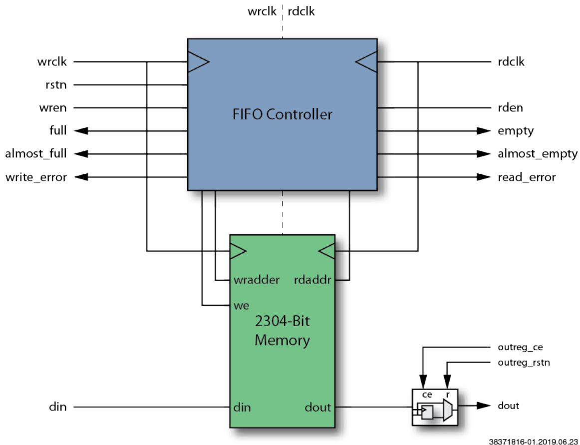
**Figure 66: LRAM2K\_FIFO Block Diagram**
