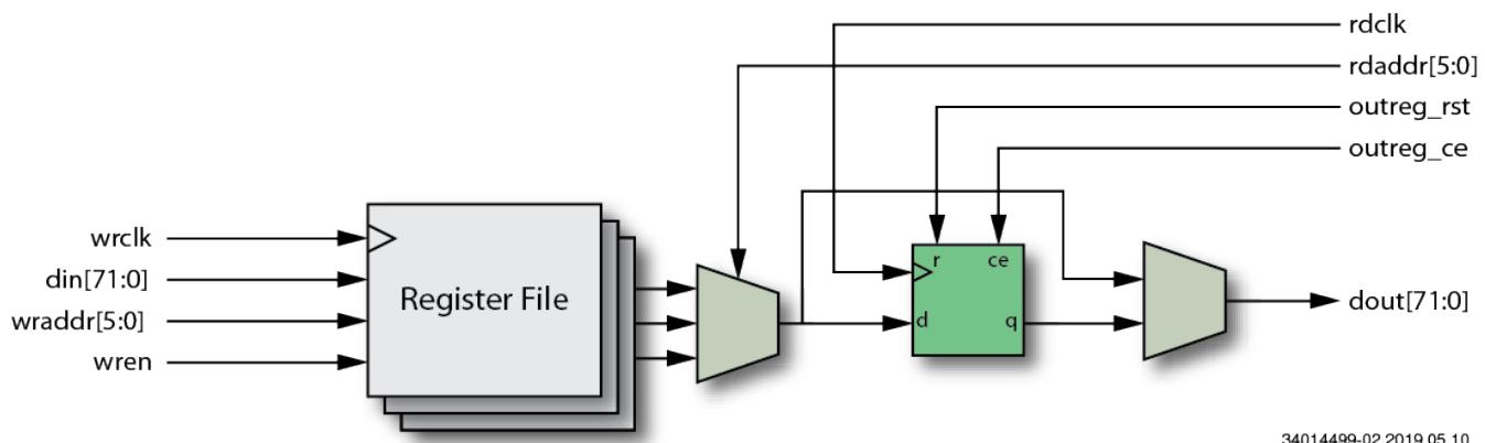
**Figure 68: LRAM2K\_SDPI Block Diagram**
