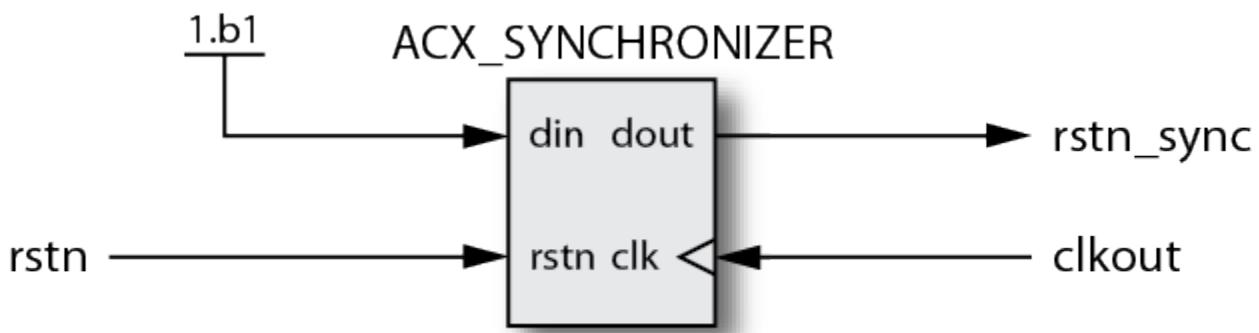
**Figure 26: ACX\_SYNCHRONIZER Logic Symbol**
