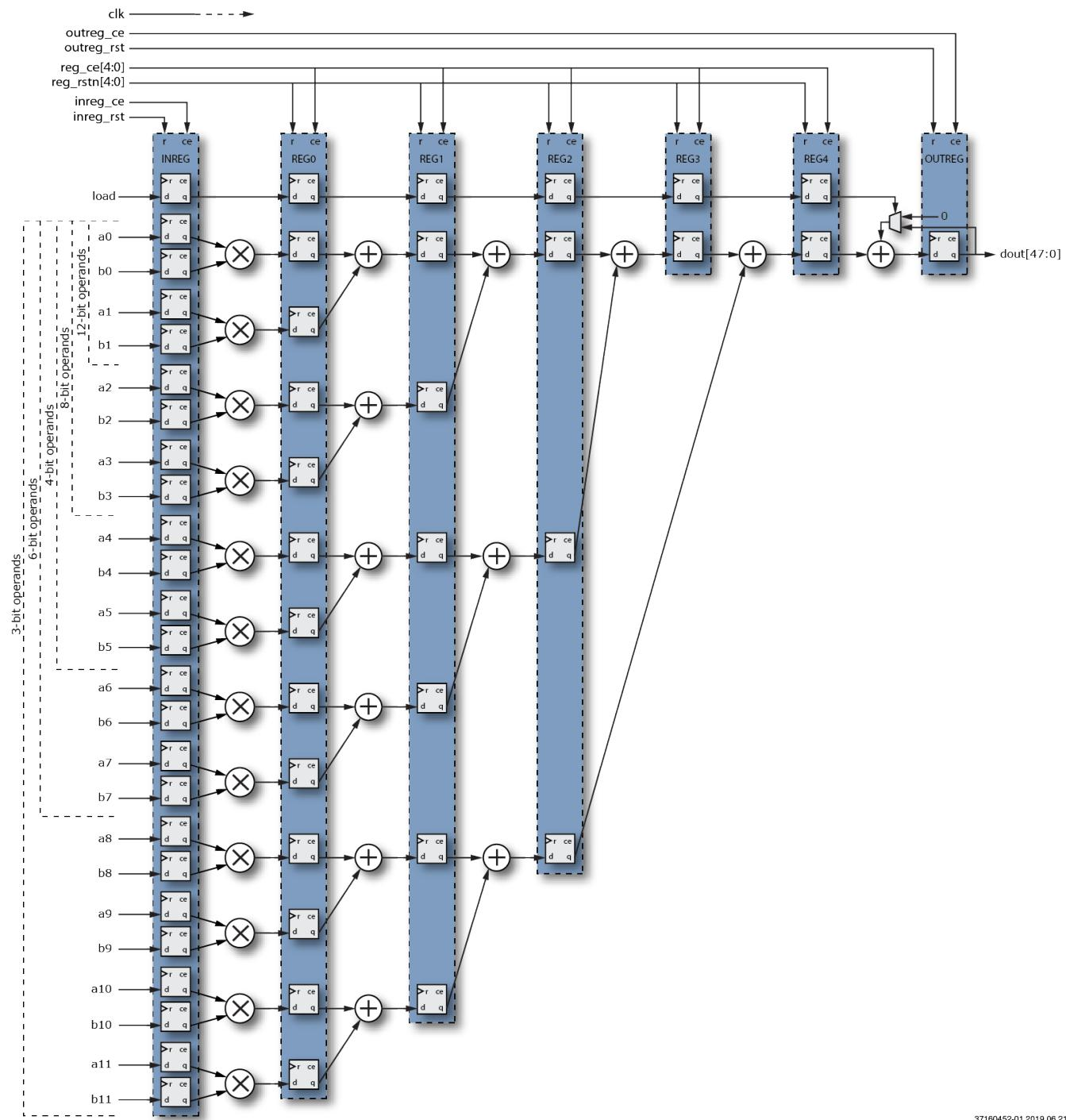
**Figure 49: MLP72\_INT Block Diagram**
