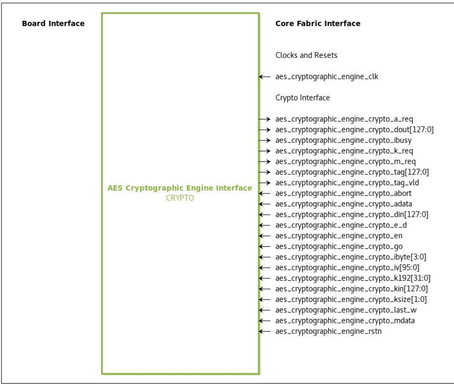
Figure 15: Block Diagram for the Speedster7t AC7t800 Cryptographic Engine
