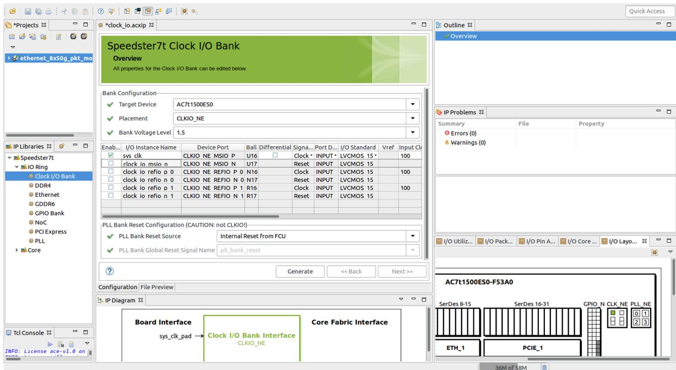
**Figure 17: Clock I/O Configuration in ACE I/O Designer**
