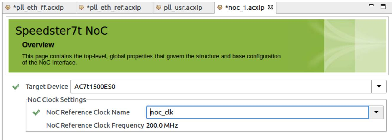
**Figure 19: NoC IP Configuration in ACE I/O Designer**
