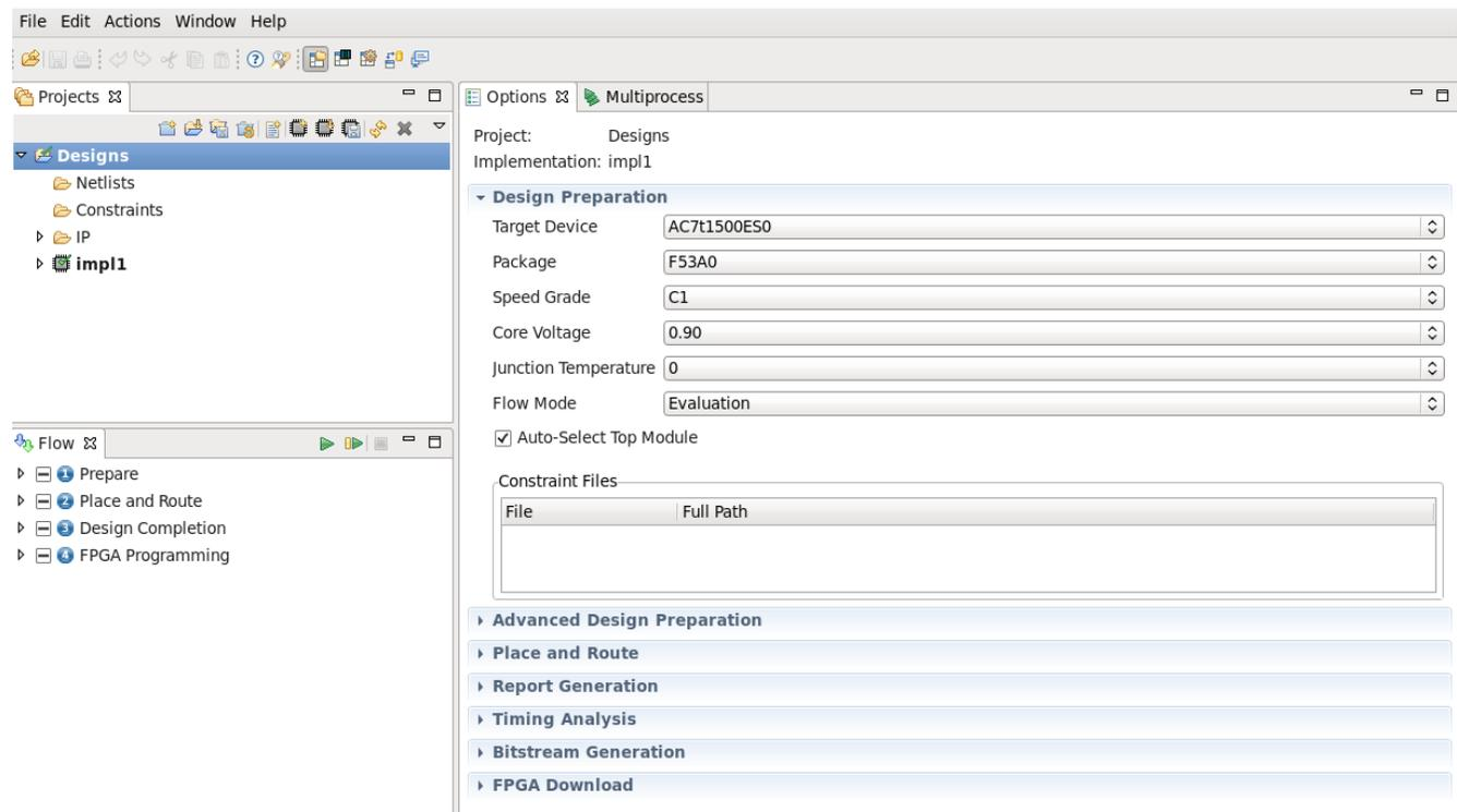
**Figure 16: Design Preparation Options in the ACE Project**
