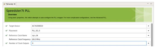
Figure 16: Number of Clock Outputs Example
