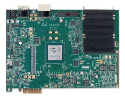
The Speedster22i HD1000 development kit from Achronix contains the world's first 22-nm programmable logic device — the HD1000, which is produced in Intel's 22-nm fabrication facility. The HD1000 development kit is optimized for development of networking and communication sub-systems — with 100 Gbps throughput, and offers the appropriate ports and memory capacity for these functions.
