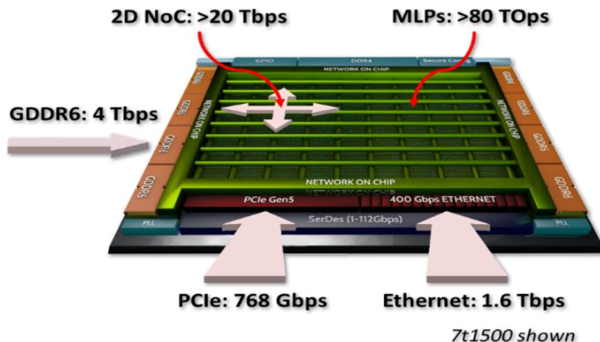
**Figure 3: Achronix Speedster AC7t1500 High-Performance FPGA Architecture**
