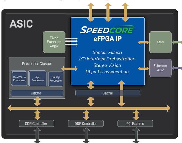
**Speedcore eFPGA IP for Custom SoC Reprogrammable Hardware Acceleration**
