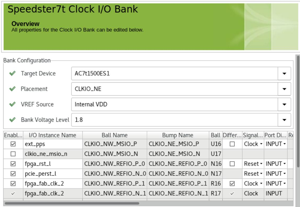
**Figure 1: Speedster7t Clock I/O Bank IP File in ACE GUI**
