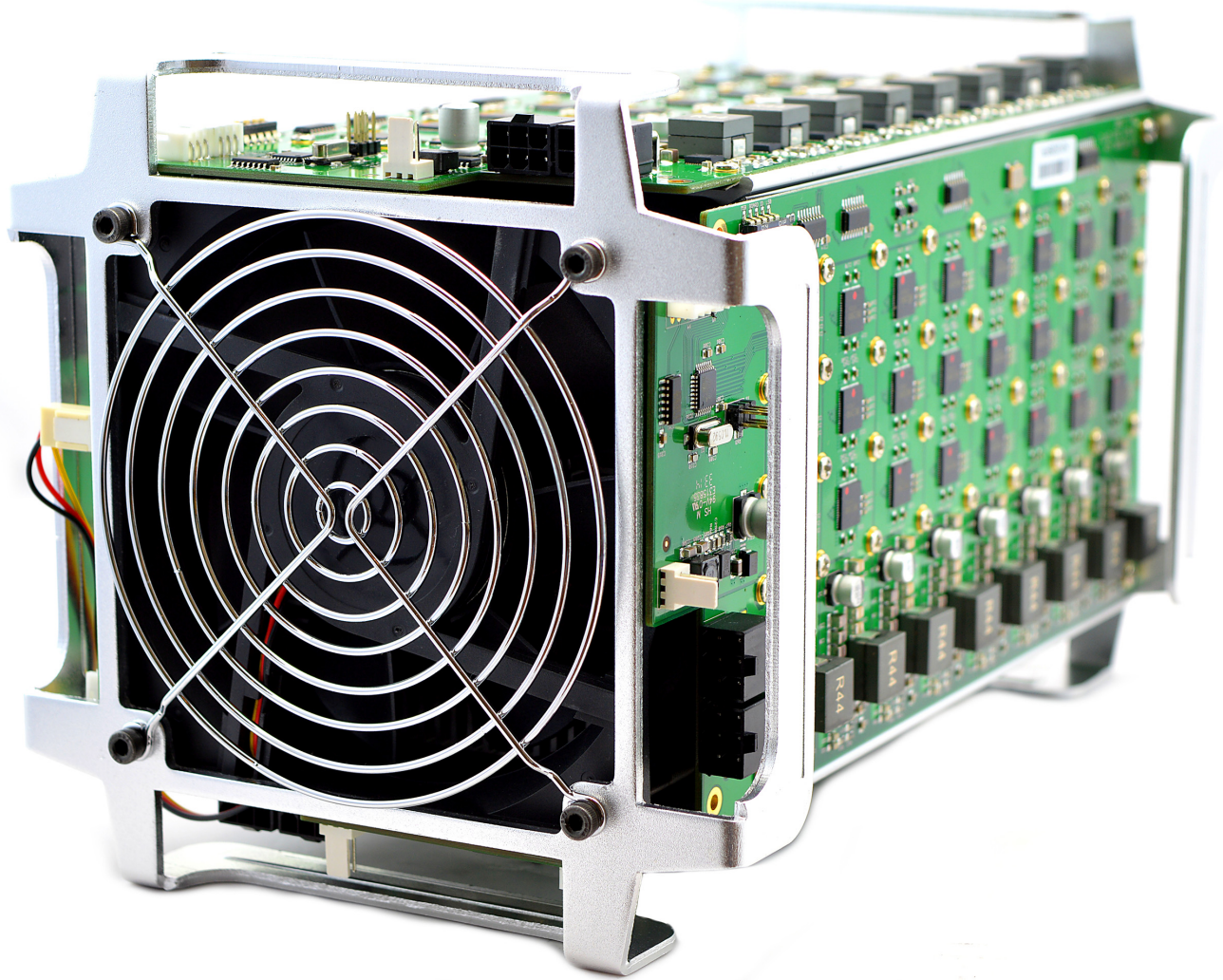
Figure 3: Bitcoin Mining Rig Enclosure. Most Popular Mining Rigs Have a Similar Form Factor
