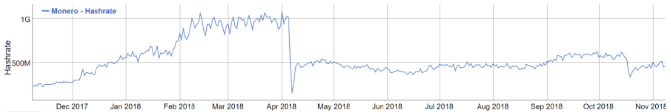
Figure 5: Global Monero Hash Rate Plotted Over Time. The fork from Cryptonight V0 to V7 in April 2018 caused a sharp drop because all non-programmable mining hardware became worthless. The next fork happened six months later as scheduled. Source: bitinfocharts.com
